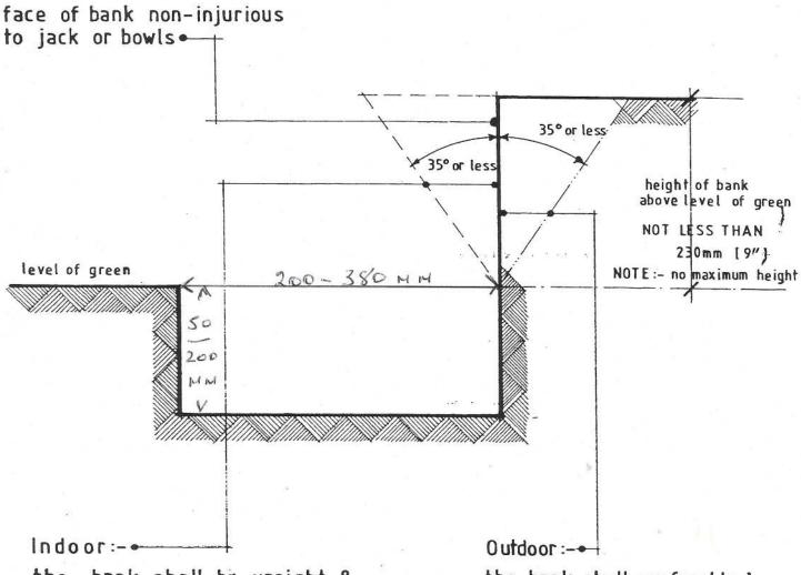
the bank shall be upright & perpendicular to the green playing surface with a tilting fillet, or alternatively the bank should be at an angle of not more than 35° from the perpendicular inclined towards the green
